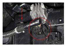
2. Access your factory fog lights. Unplug the fog lamp connector and free the harness from the retaining clip using a flathead screwdriver.
