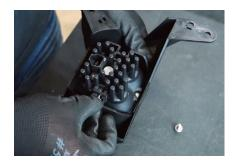
1. Install the supplied nuts into the pod housing with the nylon facing inward. Attach the bracket to the pod using the supplied screws and washers. See diagrams above. The screws will also determine the aim of your SS3 pods. Ensure that the screws are tightened such that the pod retains its position, but can pivot with force for aiming.
