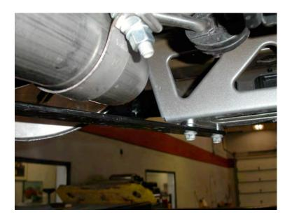
8. Install ¼" thick stainless steel spacers (SPCR\_CA10\_1), one for each side, between cross brace and bottom of the car and tighten the (4) 15 mm bolts. (This is the brace that runs directly under the X-pipe). Tighten and adjust as needed. Make adjustment so that X-pipe is situated above the cross brace by approx ½" to ¾" after tightening. See picture below.
