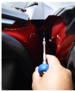
Turn the wheel all the way and pull back on the splash guard. You will need a long extension on the passenger side. You will have to go behind the windshield washer reservoir to get to the bolt securing the fender to the apron.
