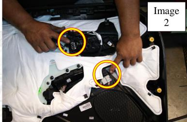
You will need to remove the speaker from the door. Once the door panel is off the door, remove two clips as shown below this will give you the extra wire slack needed to allow the door to be raised up. Also remove the tape that holds the wire harness to the inner boot on the door side this will allow the wire harness to move freely.
