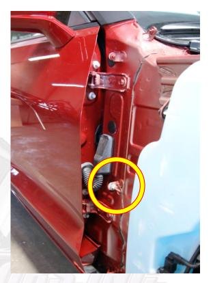
Before removing the factory hinges you MUST mark the factory location of the door on the vertical and horizontal planes. Also mark and measure the distance between the apron and the edge of the door by the top and bottom hinge.
