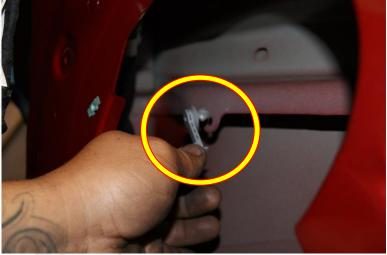
With the speaker out of the door you will now be able to remove the "Door Catch" by removing the 3 bolts securing it. It will need to be removed through the speaker hole.
