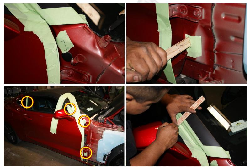
Place tape around the door and body of the vehicle as shown to help you locate the factory location. Then use 2" painters' tape to secure the door to the body.
