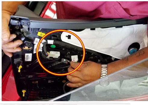
Remove the speaker by removing 4 screws. (Circled Below)
