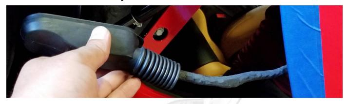
Cut the rubber wire boot in half as shown.
