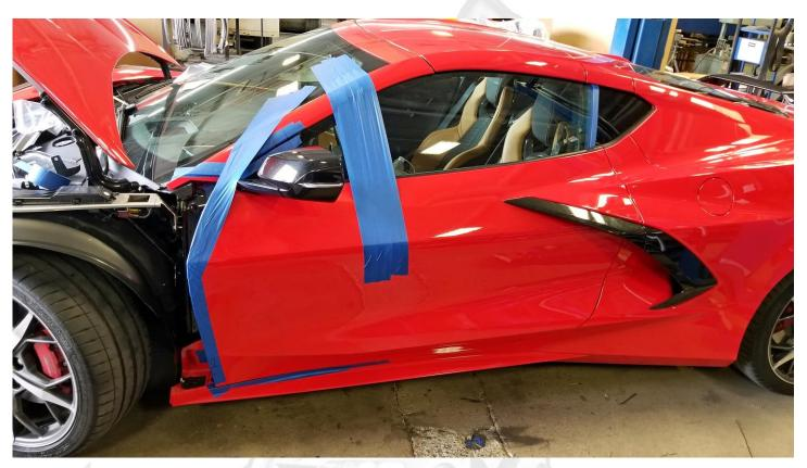
Tip: Cut a couple 3-inch pieces of paint stick to use as shims so the door does not move when you remove the factory hinges. Use them under and behind the door. Wrap them with painters' tape to get the exact thickness you need to shim the door.
