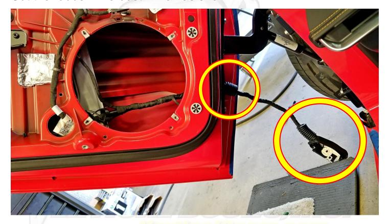
Secure each end of the boot around the wires with a zip-tie so that it is watertight as shown to the right.
