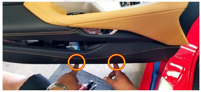
Remove the panel by pulling on it to release the clips. Then disconnect both electrical connectors.
