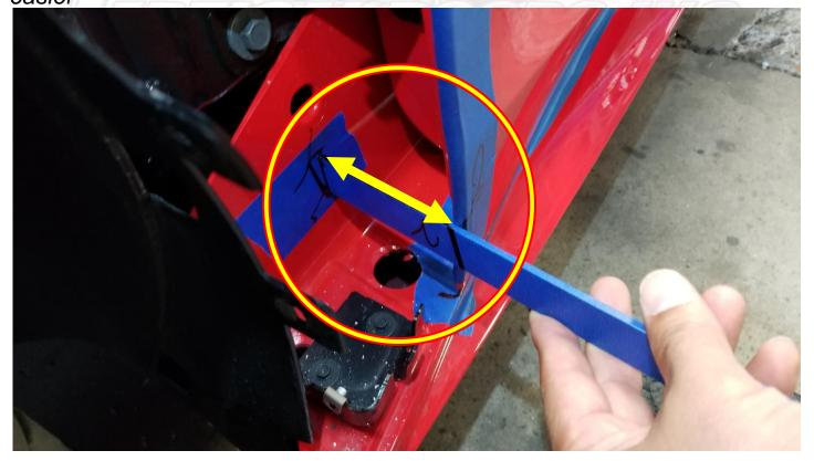
After you have marked the door location, secured the door to the body, and installed the shims, you can then remove the factory hinges and install the VDI Hinge.
