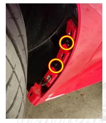
Pull back the liner and remove the bolt holding the fender. (circled to the right)
