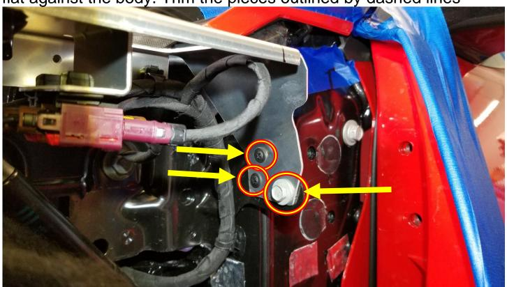
Add 2 self-tapping screws as shown above (To re-enforce the part once you trim it) Remove the circled bolt to the right of the bottom screw.
