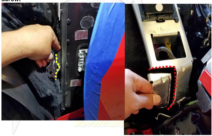
You will need to remove the door panel and the speaker to be able to remove the door catch. Two nuts secure it from the door jamb side.
