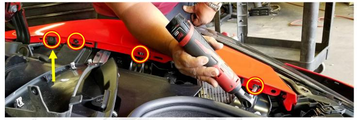
3 screws on top and 1 plastic fastener (Arrow)
