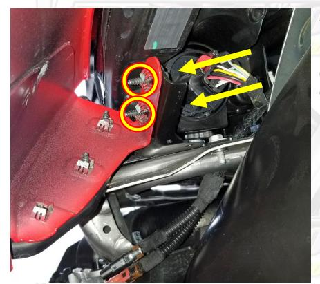
2 bolts on the inside holding the front portion of the fender (accessed from the direction the arrows are pointing)
