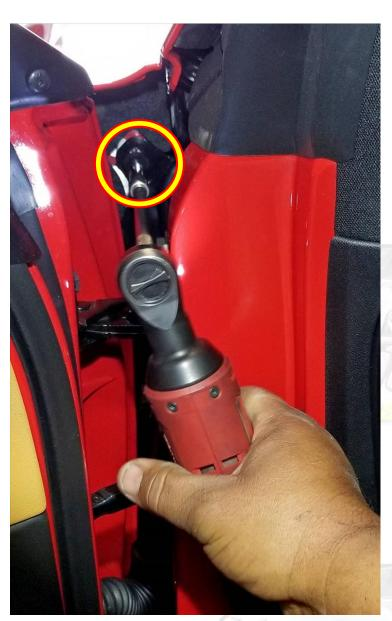
Remove 1 fender bolt (circled left) with the door open.
