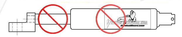
WARNING! THE USE OF ANY TYPE PLYERS, PAINT OR FOREING MATERIALS ON THE SHOCK'S BODY OR SHAFT WILL VOID THE WARRANTY.
