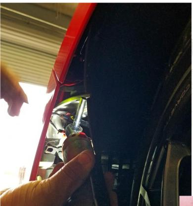
Remove the hidden bolt from the inside holding the bumper on each side as shown above and removed to the right
