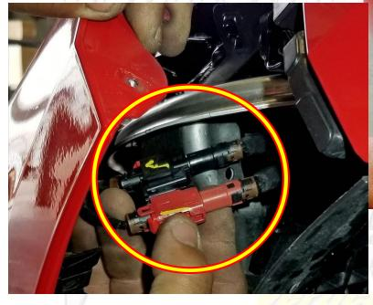
When removing the bumper, carefully unplug all wire harnesses attached to it. (Connectors: 2 on driver side, 1 on passenger side)
