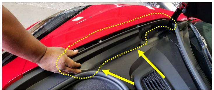
Remove the side trim pieces on each side covering the fender bolts first by pulling on them.
