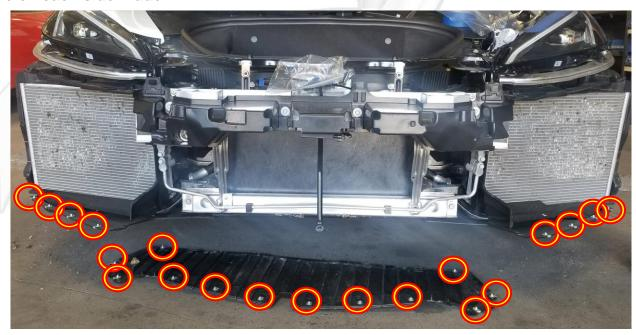
You will need to remove all the fasteners under the front bumper to be able to release it
