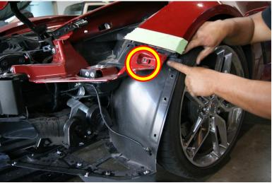
You will need to un-clip the splash guard by pulling on it towards the front of the car. Then you can Remove all the screws from around the wheel well.
