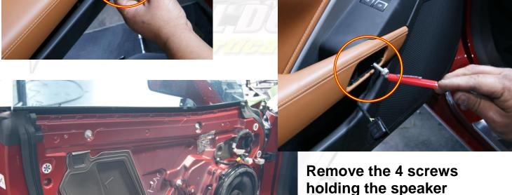
Remove all Screws holding the door panel around the edge
