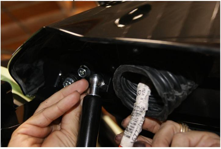
**Adjust the Hinge:** Use an Allen wrench and open-end wrench to make the first adjustment. First loosen the jam nut then turn the Allen wrench. Once adjusted properly, hold the Allen wrench and tighten the nut. This will allow you to make the striker close like factory by moving the back of the
