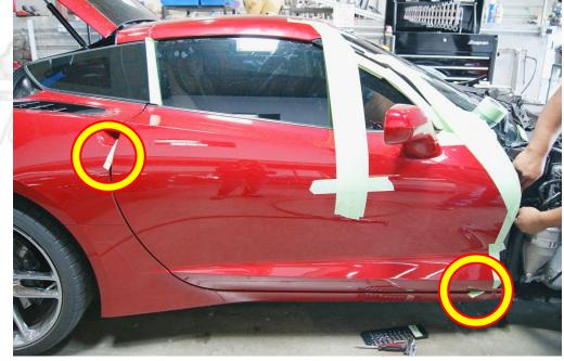
After you have marked the door location, secured the door to the body, and installed the shims, you can then remove the factory hinges and install the VDI Hinge.
