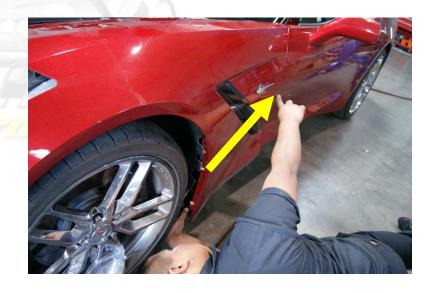
Open the door and remove the bolt securing the fender to the body as show.
