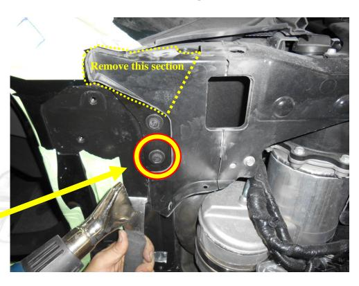
On the passenger's side you will want to remove the ECU to give you more room to work before you trim the fender bracket and install the new VDI Lambo Door hinge.
