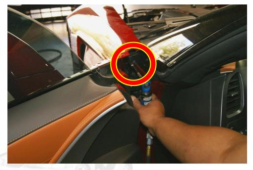
Remove all the plastic brackets and the rest of the bolts securing the fender to the body.
