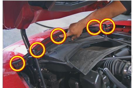
Remove all the bolts and plastic clips securing the bumper to the body and fenders
