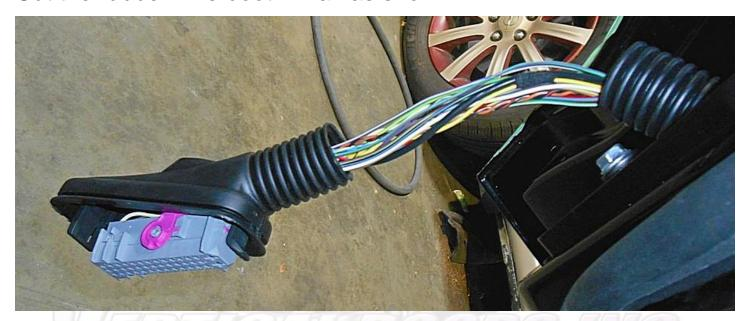
Use friction tape / cloth wire loom tape to protect the exposed wires. If you use regular electrical tape, the wires will not retain their shape and will end up getting pinched between the door and the fender. If you use wire loom it must be stretched tight over the wires and be sure to use the smallest diameter possible.
