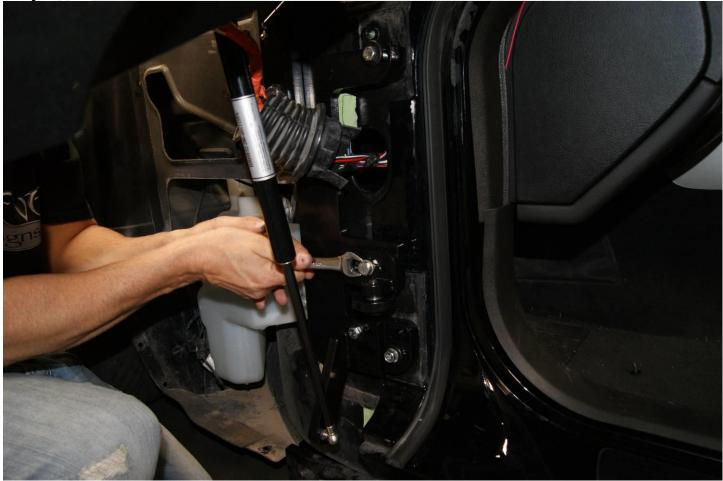
With the door closed, Loosen the bolt and slide the adjuster forward/back so that the wheel is about 1/16" from the hinge.
