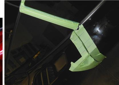
Make sure to measure and mark the distance between the body and the outer door skin at the front of the door by the bottom and top hinge as shown to the right.
