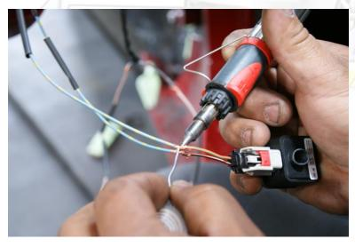
In the image we have removed the sensor to show how to extend the wires but you do not have to remove the sensor, just unplug it.
