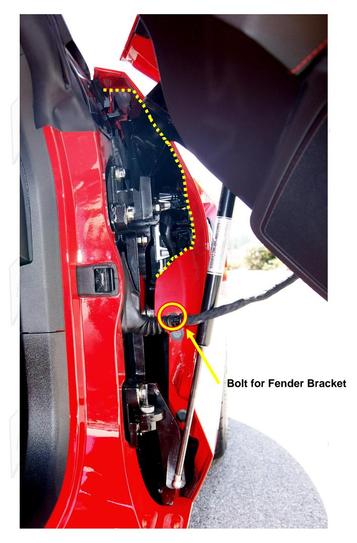
Drill new hole for support bracket...use the M6x1.00 bolt and threaded clip
