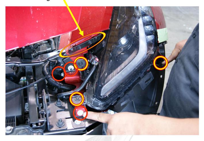
Remove all the bolts securing the headlight to the body.
