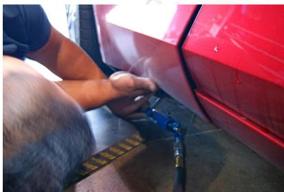
Remove the bolts at the bottom of the fender.
