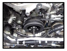
40. Install the supplied balancer hub to the stock crankshaft. Apply anti-seize to the ID of the hub and use supplied molly lube to the installer threads.
