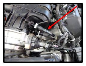
23. Remove the stock EVAP line from the hardline located near firewall and from the EVAP solenoid. Remove the (2) fittings from the factory hose (do not damage oring on fitting). *Note:* These fittings will be reused.
