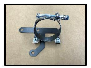
61. Install the pump mount bracket to the factory passenger side brace using the supplied (3) 8mm x 16mm HHFCS and the (3) 8mm flanged nuts on the back side. Install the IC pump into the clamp using the supplied rubber strip. Face the inlet barb up, electrical connector down and the outlet barb towards the driver side.
