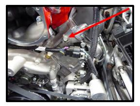
71. Install the supplied smooth and grooved 10-rib idler pulleys to the factory water pump with the snap ring facing the engine/water pump. Use the (2) 10mm x 50mm SHCS to secure with (1) 10mm step washer per pulley. Mount the supplied smooth idler pulley to the factory water pump upper location and grooved to the lower water pump location. Torque to 22 ft-lbs (15mm socket).
