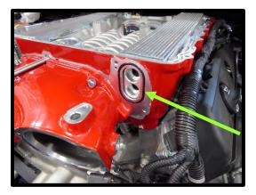
96. Carefully install the intercooler cross-over to the manifold by pushing the (4) fittings and cross-over into the intercooler cores. Orings must have grease to fit properly. Use the suppled (2) 6mm x 65mm HHFCS (top), (1) 6mm x 55mm HHFCS (driver side lower) and (1) 6mm x 45mm HHFCS (passenger side lower) bolts. Torque in 2 passes (10mm socket), first pass 65 in-lbs, second pass 75 in-lbs.
