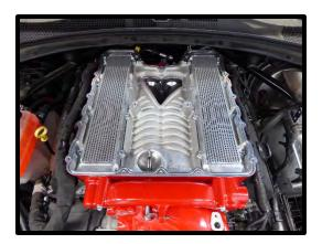
93. Install the supplied (8) 6mm x 10mm HHFCS bolts per core, apply light amount of blue #243 Loctite to threads. Before securing bolts, center the core both front to back and side to side. Torque the (16) bolts in 2 passes (10mm socket), first pass 70 in-lbs and second pass, 85 in-lbs.
