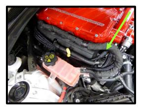
105. Secure the EVAP and driver side vent line to each other with zip-ties along passenger side valve cover, between the dipstick and passenger side vent line.
