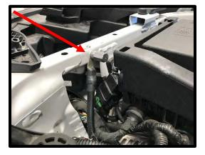
54. Remove the factory fuse box nuts, install the supplied intercooler pump relay bracket onto the stud closest to front of vehicle then the fuse holder to the passenger side stud. Secure both with factory nuts.
