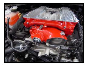
97. Install the supplied (2) black intercooler cross-over inlet/outlet fittings and mounting fork to cross-over. Apply light amount of grease to orings for proper installation. Use the supplied (1) 6mm x 10mm HHFCS to secure mounting fork. Torque in 2 passes (10mm socket), first pass 70 in-lbs, second pass 85 in-lbs.
