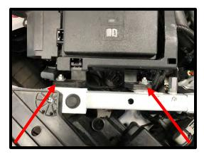
55. Route the 2-way EVAP connection towards the front passenger side of the engine for later connection. Route the intercooler pump 4-way down between the radiator and frame for later installation.
