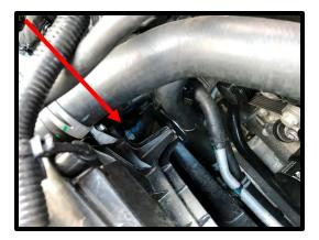
50. (Auto transmission) Reinstall the retaining clip to secure the transmission cooler line to the radiator.
