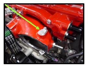
87. Install the supplied PCV hose from the valley cover PCV valve to the bottom 6 ORB fitting on the odd cylinder side of inlet.
