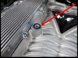
99. Install (2) of the (13) supplied 6mm x 30mm HHFCS in the back 2 bolt holes. Install lid to the manifold by sliding under the cowling. Secure lid to manifold using the (13) 6mm x 30mm HHFS on the perimeter then the (5) 6mm x 40mm HHFCS on the inside. Torque in 2 passes (10mm socket), first pass to 75 in-lbs and second pass, 96 in-lbs.
