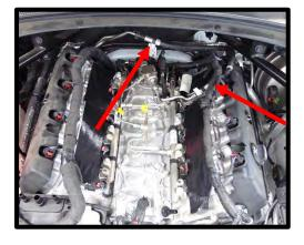
76. Cut a 6" section of foam from the factory driver side valve cover vent line. Install the foam piece to the factory EVAP tube where it is closest to the factory fuel feed line hose to prevent rubbing together. Secure both ends with zip ties.
