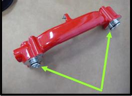
95. Install the (2) orings on the manifold to intercooler cross-over surface on the front of the manifold. Use light amount of grease to help secure oring in place.
