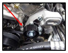
74. Install the grooved idler pulley with the 10mm step spacer through the front of the pulley, .250" step spacer on the back, then the 10mm sliding tee-nut at the back of the tensioner bracket. Use the (1) supplied  $\frac{1}{2}$  x 2  $\frac{1}{4}$ " HHFCS to secure assembly. Leave loose now for proper belt installation.
