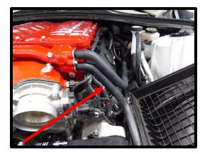
114. Install the supplied formed hose (#3102529) from the IC cross-over upper (outlet) fitting to the filler neck back fitting. Secure both ends with supplied pinch clamps.
