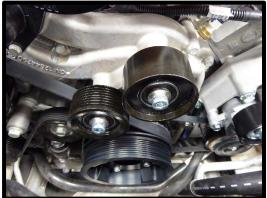
72. Install the supplied tensioner bracket to factory odd cylinder side block and cylinder head using the supplied (2) 10mm x 100mm HHFCS and (2) 8mm x 60mm HHFCS. Torque M10 bolts (15mm socket) to 32 ft-lbs and M8 to 22 ft-lbs (12mm socket).
