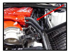
115. Secure the previously routed reservoir feed and vent line to the front fittings on the IC filler neck. Secure with supplied pinch clamps.
