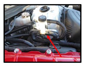
113. Secure the previously routed LTR outlet hose (LTR outlet) to the lower (inlet) fitting on the IC cross over. Secure with supplied pinch clamp.
