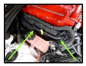
104. Connect the previously routed 3/8" x 53" vent line from driver side valve cover to the inner fitting on catch can.
