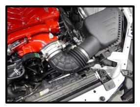
119. Install the supplied 9.89mm to 3/8" barb fitting to the supplied 90deg inlet tube.
