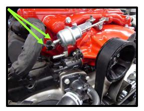
102. Connect the 3/8" x 45" EVAP hose previously routed (straight fitting) to the EVAP solenoid.
