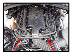
14. Using a clamp tool, remove the sound tube from the inlet elbow.
