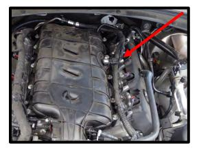
27. Using a 10mm socket, remove the (10) bolts securing the intake manifold to the cylinder heads. Carefully remove the intake manifold assembly and foam valley insulator.
