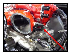
88. Install the original EVAP line fittings to the supplied 3/8" x 45" EVAP hose. Apply light amount of grease to oring to help ease installation.
