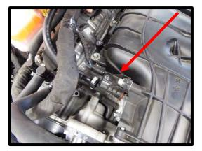
25. Disconnect the factory brake booster line at the check valve junction.
