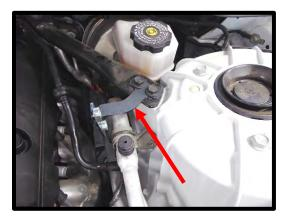
112. Mount the filler neck to the bracket using the supplied (2) 6mm x 12mm BHFCS. The vent line should face forward.
