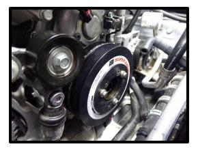
43. Using a stretchy belt installation tool and install factory stretchy belt onto new damper and A/C compressor. NOTE: Be careful not to damage belt. Inspect the belt for any damage after the installation.
