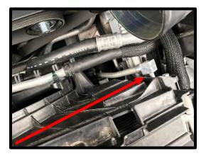
35. (Auto transmission) Using a panel puller tool, remove the coolant lines from the fan shroud.
