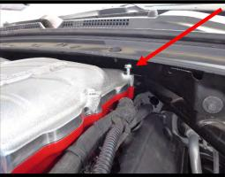
100. Install the bypass actuator to the cross-over using the (2) 8mm x 12mm BHCS. The bypass holes are slotted, therefore before securing bypass, slide the bypass towards centerline to pre-load the actuator arm. Once pre-load is set, torque bypass bolts to 15 ft-lbs (5mm allen socket).
