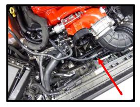
121. Refill the Engine coolant. Verify that your coolant drain is closed, and use a filter/strainer to pour the recycled coolant/water mixture that you drained from the radiator. If necessary top off with a **GM approved engine coolant**. Whipple also recommends running 2 bottles of Redline Water Wetter which can be found at most automotive parts stores.
