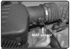
**10.** Using T25 torx bit, loosen and remove the 2 screws holding in the MAF sensor and remove from OEM intake tube.
