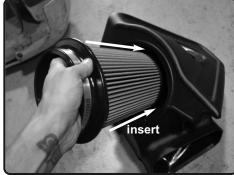
**8.** Install the filter into the air box housing. Position the Twist-Lock™ filter pattern to the hole cut out on air box.
