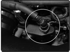
**17.** Re-connect the crank case line to the fitting on the intake tube. Make sure you hear the click to make sure its secured.
