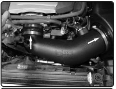
**15.** Install the intake tube into the vehicle. Position the intake tube to the throttle body and filter. Adjust and tighten clamps.
