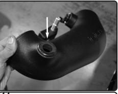
14. Install the large grommet to the hole on the intake tube
