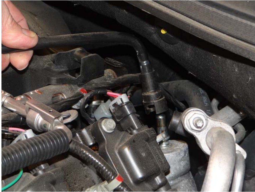
Step 4: Remove PCV line from valve cover.
