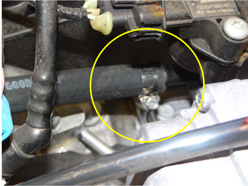
Step 12: Install hose over intake nipple.
