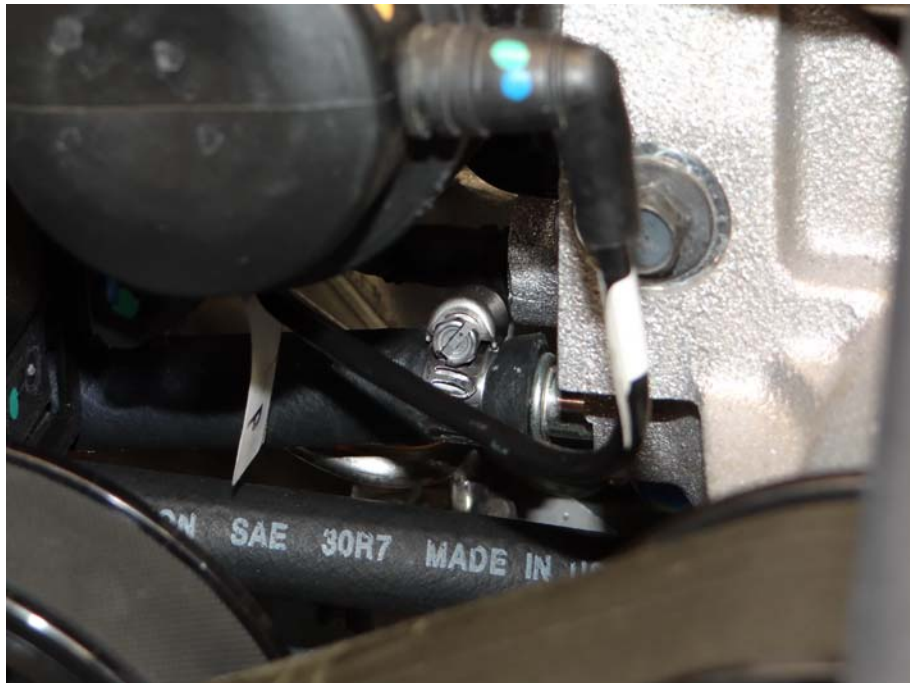
Step 7: Install hose over intake nipple and tighten hose clamp.
