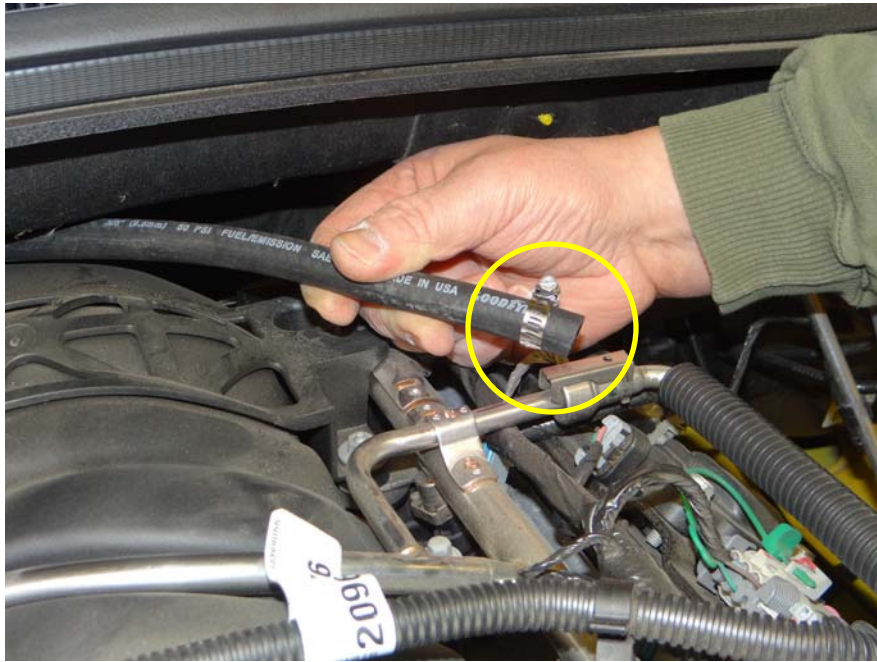
Step 8: Install hose clamp.
