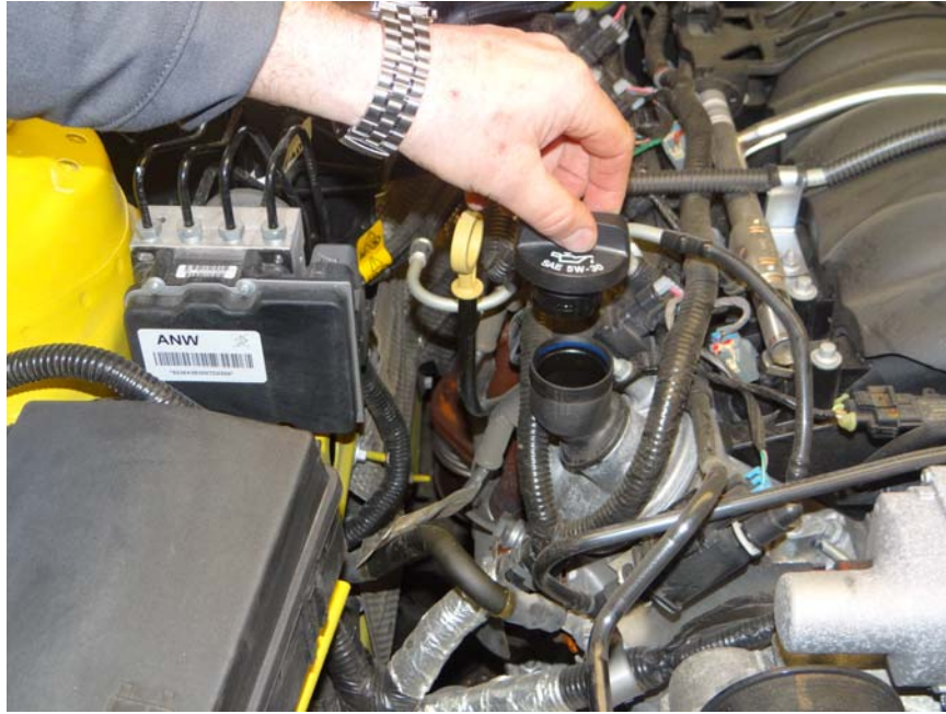
Step 2: Re-install oil fill cap.
