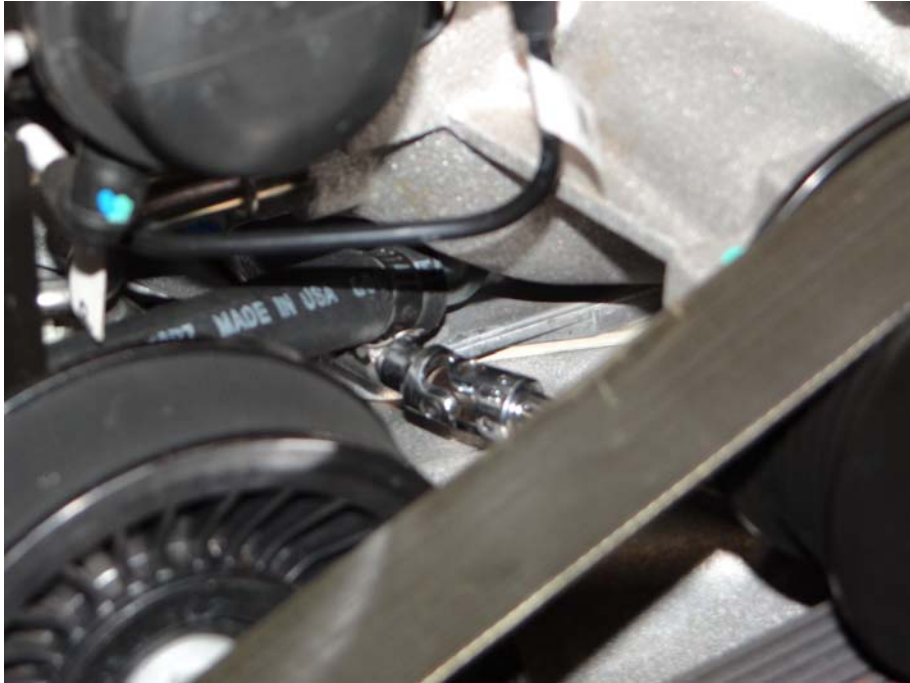
Step 4: Install hose over lifter valley nipple and tighten hose clamp.
