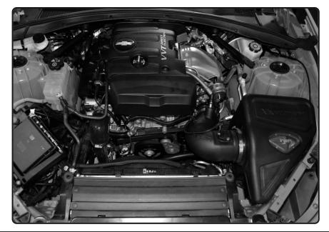
Congratulations! You have just completed the installation of this intercooler pipe system. Periodically, check the alignment of the intercooler pipes, normal wear and tear can cause nuts and bolts to come loose. <u>Note: Check</u> <u>clearance and adjust if needed! Failure to check the alignment and adjust the intercooler pipes can cause</u> <u>damage that will void the warranty. Injen Technology is not responsible for any damages caused by/from</u> <u>improper installation.</u>
