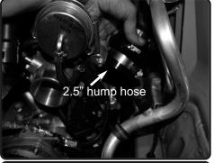
**27.** Once the machined fittng is secured into place, install the provided 2.5" hump hose with clamps provided to the intercooler pipe. Secure on intercooler pipe and tighten clamp.
