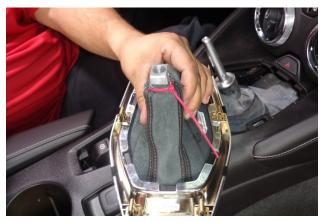
6. Use the supplied cable tie to secure the opening of the boot to the notch at the base of the shifter handle. Trim the excess cable tie.
