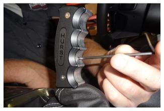
10.Install and tighten the set screw (3) in the front of the shifter handle.
