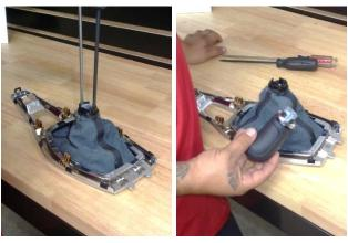
3. Use 2 flat-tip screwdrivers to separate the shift handle from the plastic collar.
