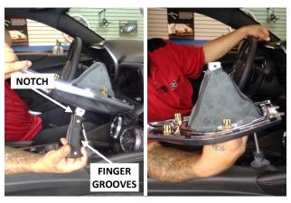
5. With the finger grooves pointing forward, work the base of the shift handle (1) through the opening in the shifter boot until the opening surrounds the notch at the base of the shift handle.
