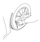
To check inflation pressure with a tire pressure gauge:
