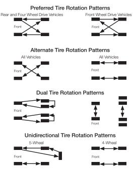
Full-size spare tires (not temporary spares) of the same size, construction, and speed rating may be used in a five-tire rotation pattern.
